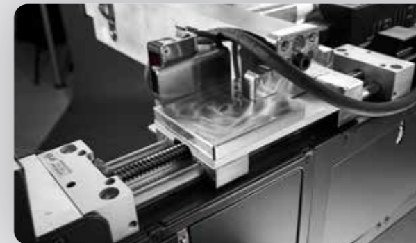
High-precision guidance of the print head towards the wall. Compensates for wall unevenness of up to 10 cm.
